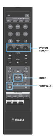
Press the ENTER key to start the AUTO SETUP procedure and then leave the room within 10 seconds.
