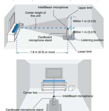
Make sure that there are no obstacles between the IntelliBeam microphone and the walls in your listening room as these objects obstruct the path of sound beams. However, any objects that are in contact with the walls will be regarded as a protruding part of the walls.
