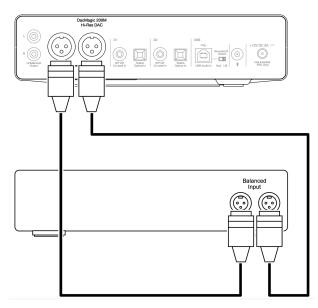
The XLR output is preferable for long connections if your amplifier features balanced XLR inputs. It can better reject noise and interference in the cable. It is possible to use the RCA phono connections and the XLR balanced connections at the same time, e.g. for connecting to different amplifiers or multi-room operations.
