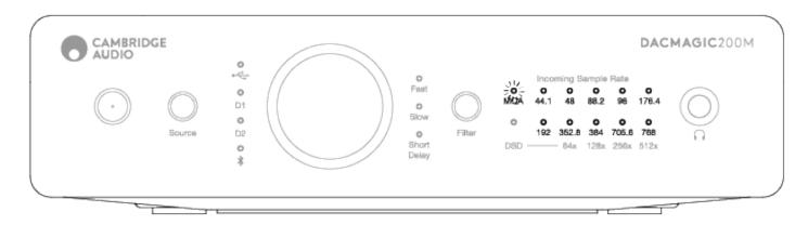
The MQA LED glows magenta to indicate that the unit is rendering an MQA stream or file. This delivers the final unfold of the MQA file.
