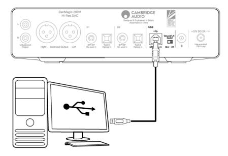
Class 2 USB Audio only. Windows based PCs require a Cambridge Audio USB driver to be installed before connection.
