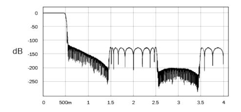
The Short Delay (minimum phase) filter is another highly regarded audio filter that offers even lower ripple in the pass and stop bands. Unlike the Linear Phase filter, group delay is not constant; however, phase shift is low and the particular benefit with this filter is that the impulse response exhibits no pre-ringing.
